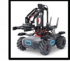
**Engineer (x1)** - *DJI Robomaster EP*Picks up and collects ammo bottles to be scanned by standards
