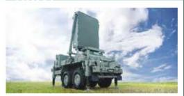
The TPQ-53 Weapon Locating Radar provides improved acquisition and identification of hostile rocket, artillery and mortar threats for early warning to enhance force protection and enable swift destruction of hostile threats.
