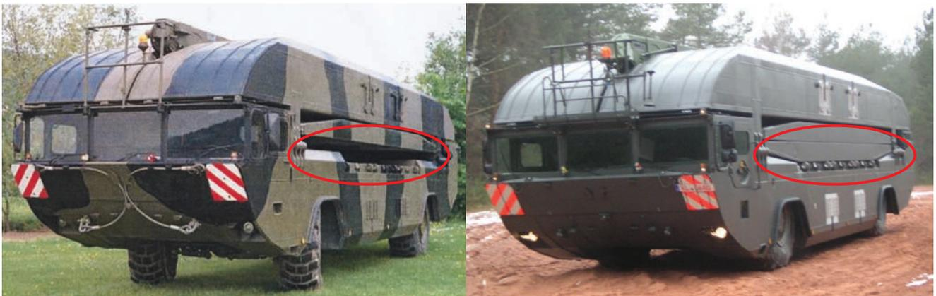
Figure 4. OEM’s M3 bridge with one ramp on the each side versus Singapore’s M3G with two ramps on each side. The third ramp on OEM’s M3 bridge is stowed in the centre of the vehicle and is not visible.
