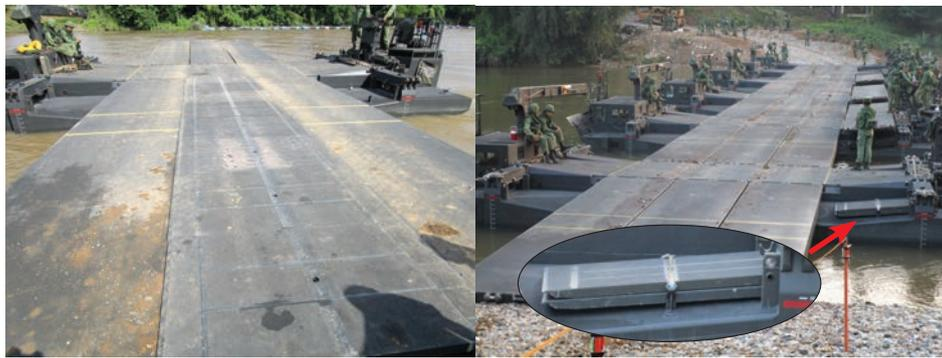
Figure 5. The modular panels of the M3G as a third ramp. The modular ramps are stored as seen on the right.
