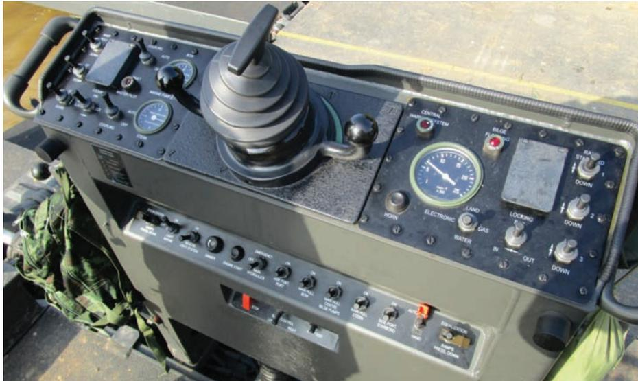
Figure 3. Demonstration of the marine controls of the M3G. The level controls the power and primary direction, and the “horns” control the relative rotation of the rig.
