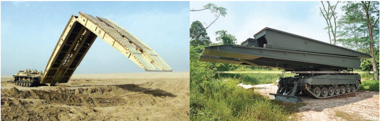
Figure 1. Scissor-launch mechanism on a M60A1 AVLB (© Quihuis / File:M60A1 Armoured Vehicle Landing Bridge.jpg / [http://www.news.navy.mil/view\\_single.asp?id=5015](http://www.news.navy.mil/view_single.asp?id=5015) / Public Domain) (left) and horizontal-launch mechanism on a Leopard 2 Armoured Vehicle Launched Bridge (Ong, 2013) (right)
