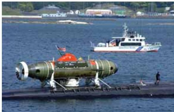
Figure 2. DSRV-1 Mystic transported on a mother submarine (Source: Undersea Warfare – the official magazine of the US Submarine Force)
