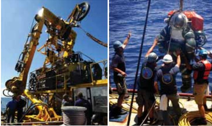
Figure 3. The SRDRS launched using its A-Frame (left) and the ADS (right)
