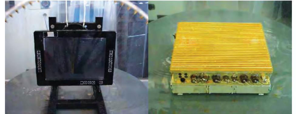
Figure 2. Spraying water test
