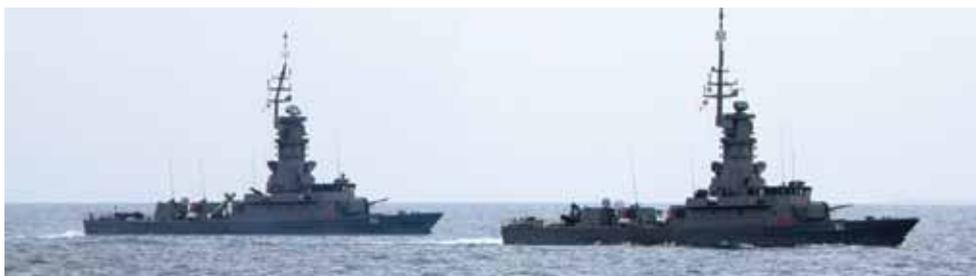
Figure 1. The pre-upgrade MCV (left) and upgraded MCV (right) sailing together. The hull and major structures remain largely unchanged, while the most observable difference is the taller and straight mast configuration where new sensors are located
