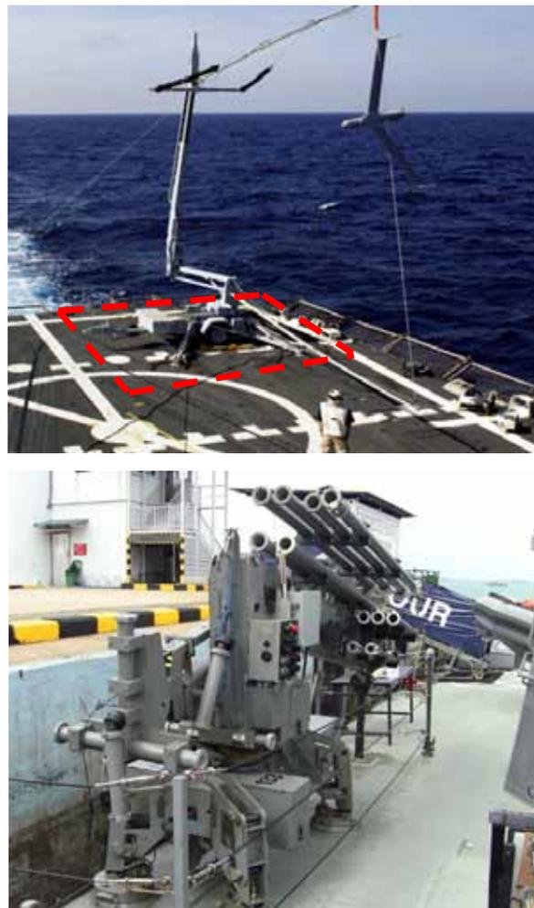
Figure 3. (a) The UAV recovery system in its original form, with its outriggers and wheels outlined in red
