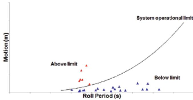
Figure 6. Sea-keeping data used to determine ship operational limit for UAV recovery
