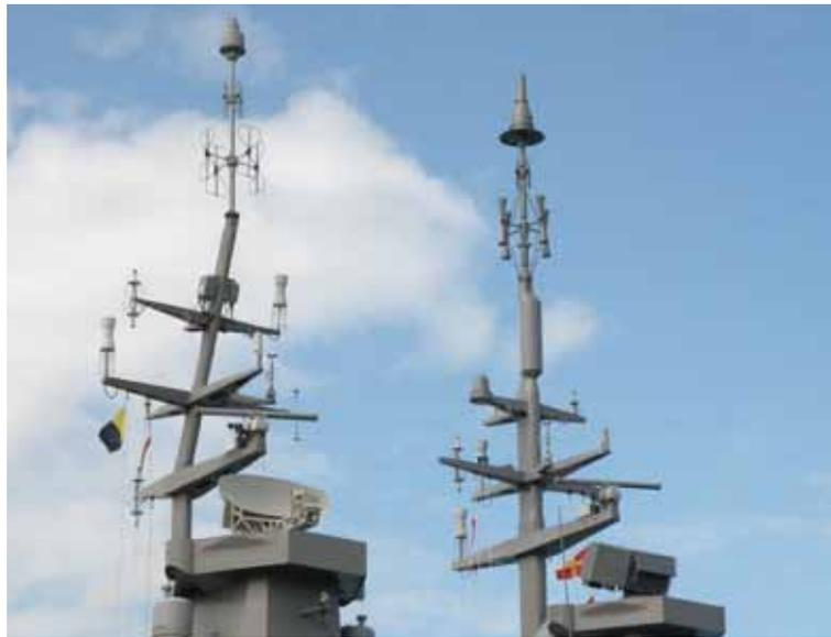
Figure 4. The pre-upgrade MCV with its slanted mast (left) as compared to the upgraded MCV with its straight mast (right)
