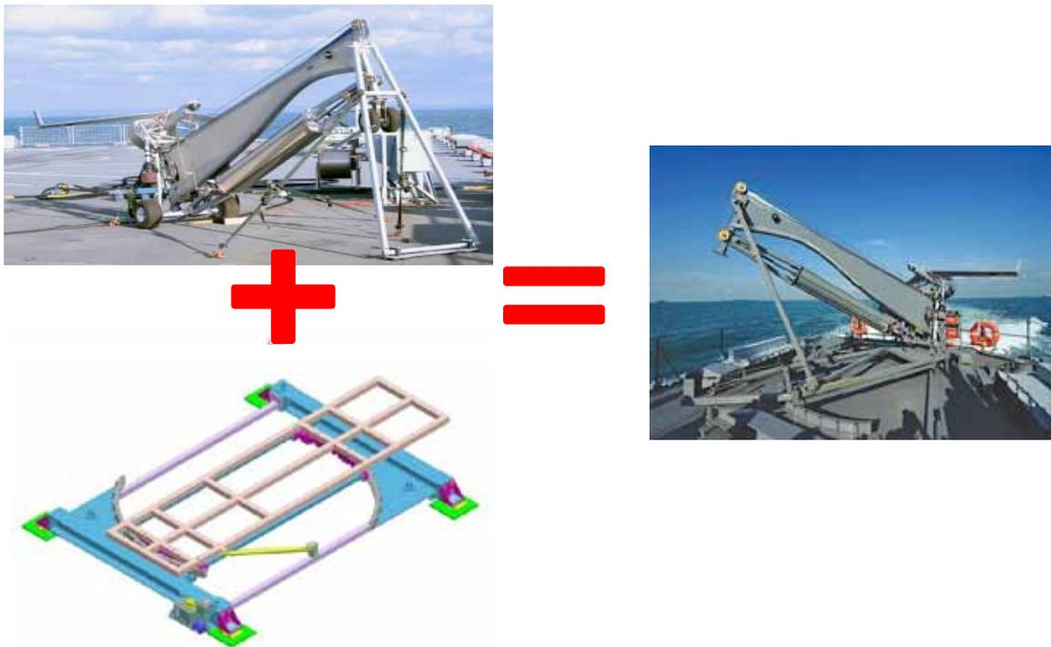
Figure 2. (a) The launcher in its original configuration and the UAV turntable concept
