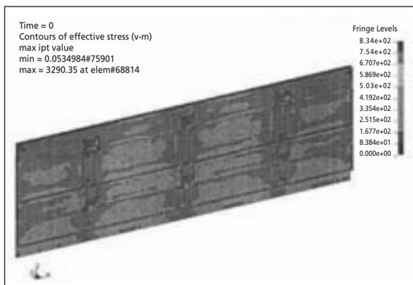
Figure 12. A Finite Element Method study made on a blast load case on a blast shield design
