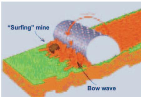
Figure 5. An example of a mine "surfing" on the bow wave
