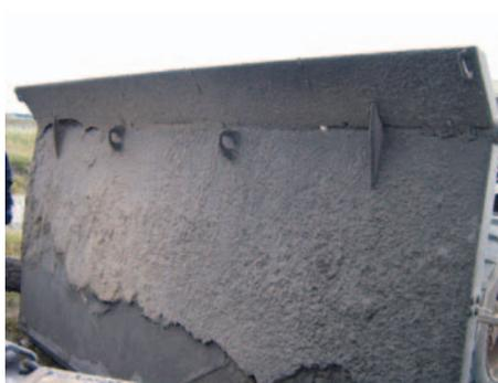
Figure 14. The blast shield from the Hydrema 910 Series 2 – the flexible flap at the top of the shield deflects the blast wave over the cab without sustaining damage from the blast wave. In addition, the tilted angle of the flap helps to recirculate dust in blast shield during flailing operations.
