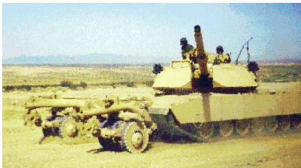
Figure 6. M1A1 equipped with mine roller
