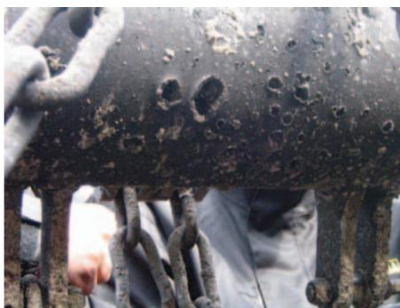
Figure 13. Fragmentation damage from an anti-tank mine with 4.45kg TNT
