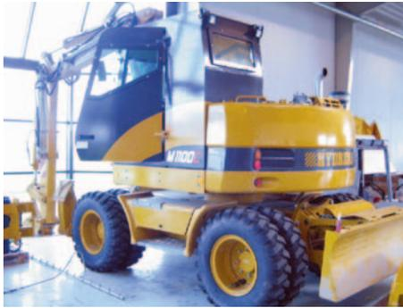
Figure 7. The Hydrema M1100 excavator with an armoured cabin which can be attached with different tools for mechanical demining
