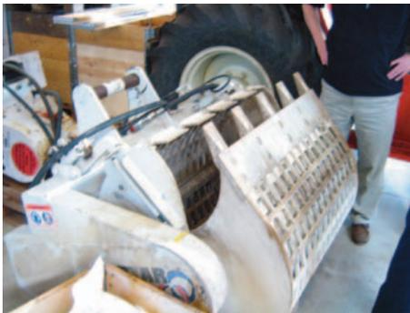
Figure 8. A mechanical sifter which can be attached to a commercial mechanical demining machine
