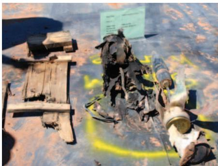
Figure 15: SAPOM in wooden crate – confined trial 2
