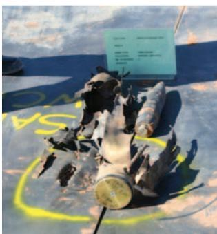
Figure 14: SAPOM in wooden crate – confined trial 1
