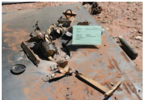
Figure 9. MOM in wooden crate – confined trial
