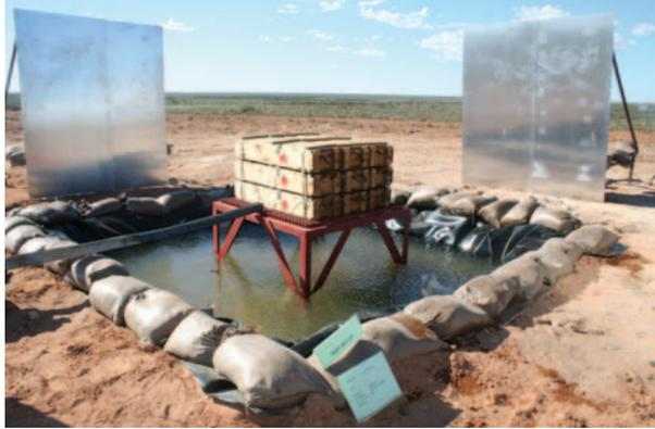
Figure 23. Fast cook-off test set-up
