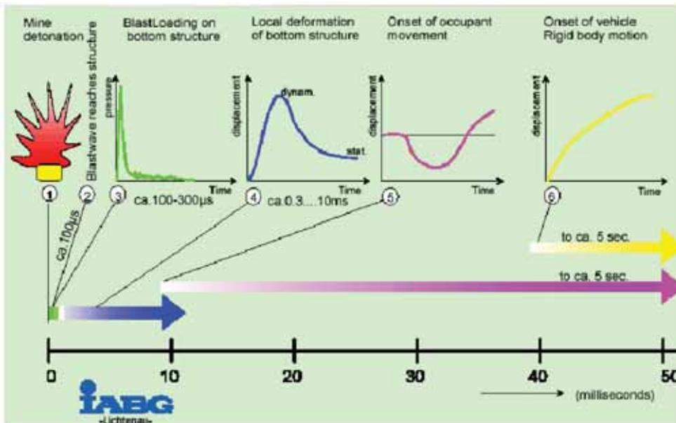
Figure 12. Effects of a mineblast on a vehicle
