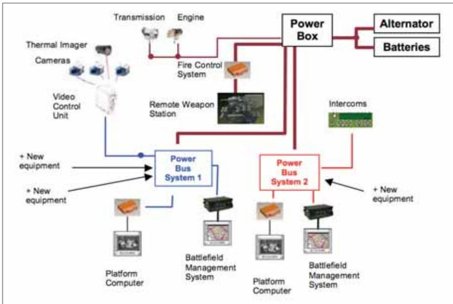
Figure 16. Intelligent power management systems architecture
