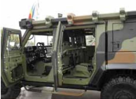
Figure 10. An IVECO 4x4 truck with AMP-ADS on the roof
