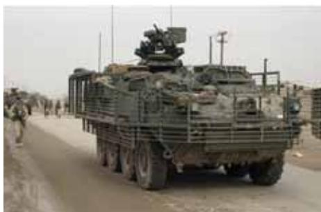
Figure 8. Slat armour on a Stryker vehicle
