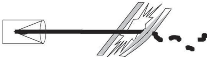
Figure 7. The disruptive mechanism of ERA
