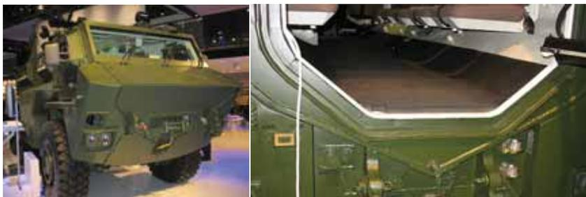
Figure 11. A RG-35 Vehicle showing a V-shaped hull
