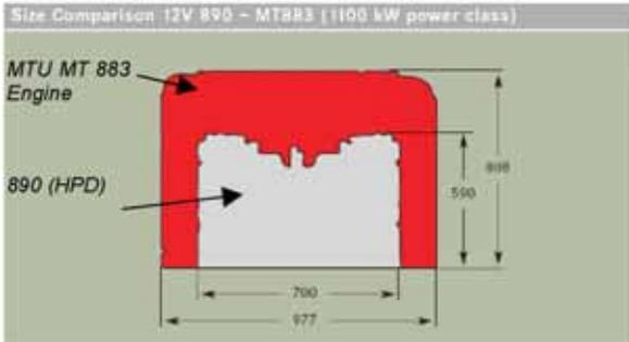
Figure 13. Comparison of MTU MT 883 and the 890 (HPD) engine sizes
