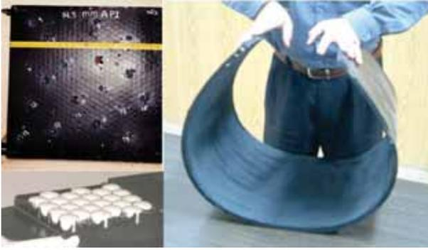
Figure 6. LIBA demonstrating its multi-hit capability and flexibility
