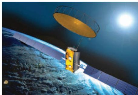
Figure 5: Mesh reflector on INMARSAT 4 satellite
