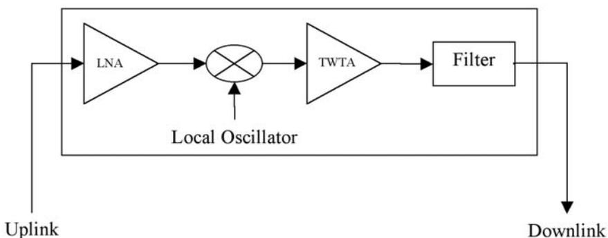
Figure 1: Schematic of bent-pipe payload (Gupta, 2003)
