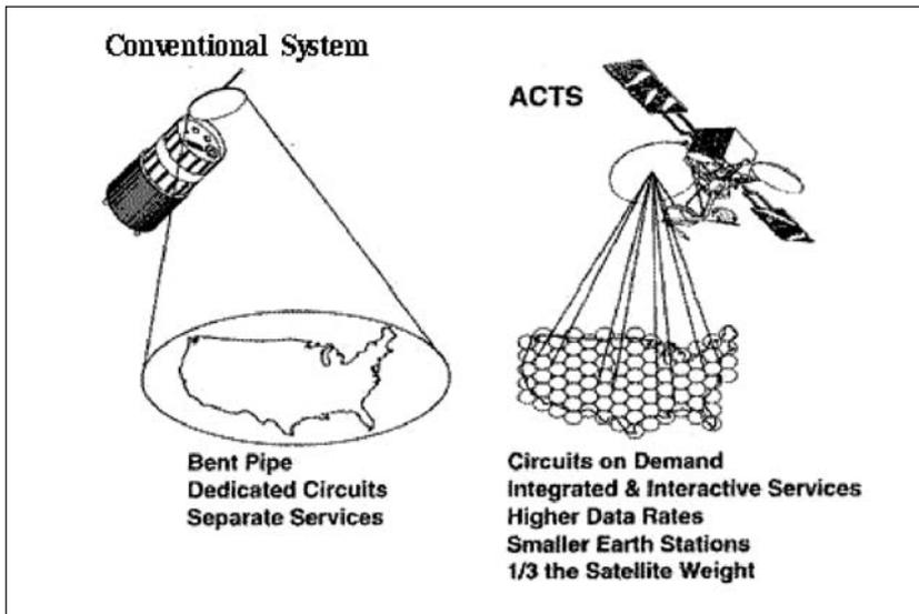
Figure 7: Multi-Beam antenna technology in the ACTS
