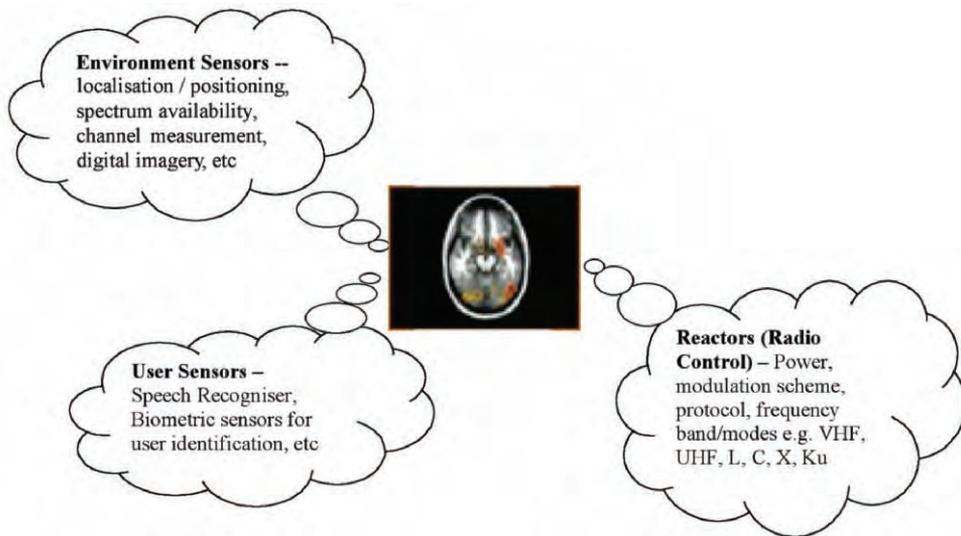
Figure 2. Potential required functionalities of a cognitive radio<sup>5</sup>
