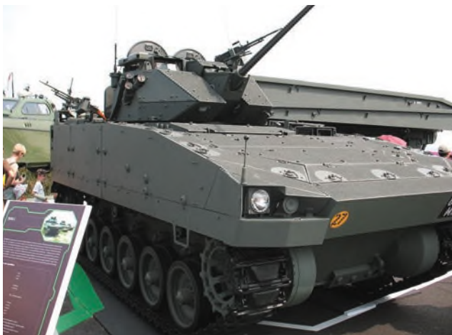
Figure 2. Modular armour of BIONIX IFV (Hazell, 2006)
