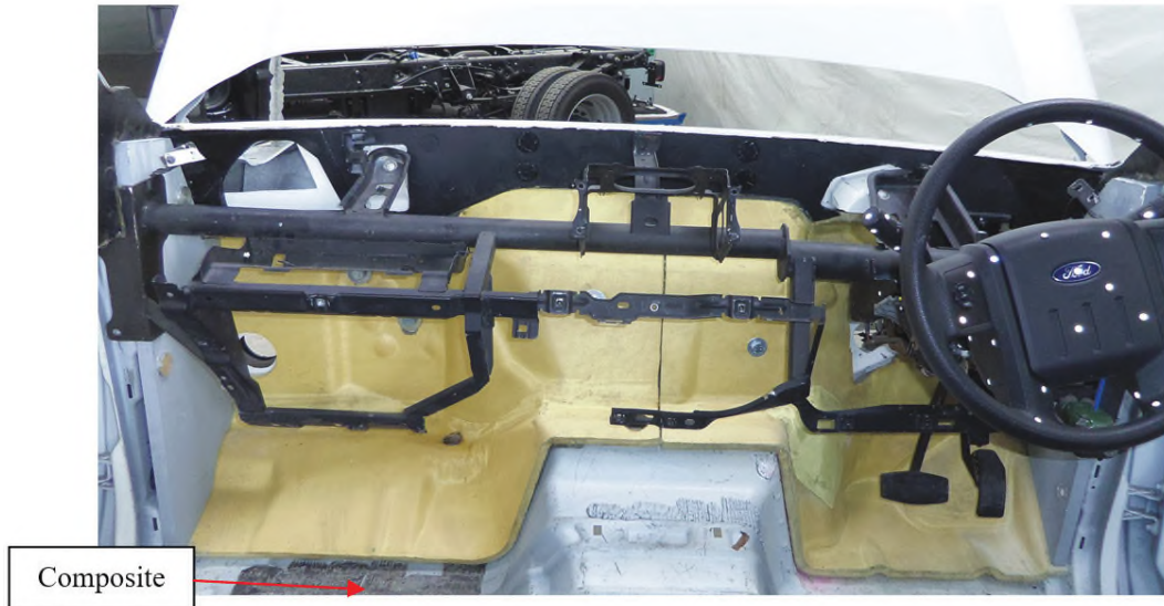
Figure 9. Composite used in an SAF project to protect the firewall of passenger compartment
