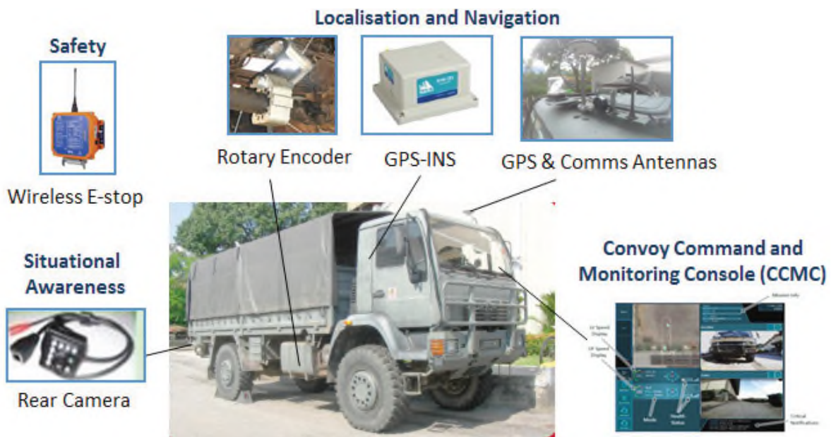
Figure 2. Main hardware subsystems installed on the Lead Vehicle (Reprinted with permission from ST Engineering)
