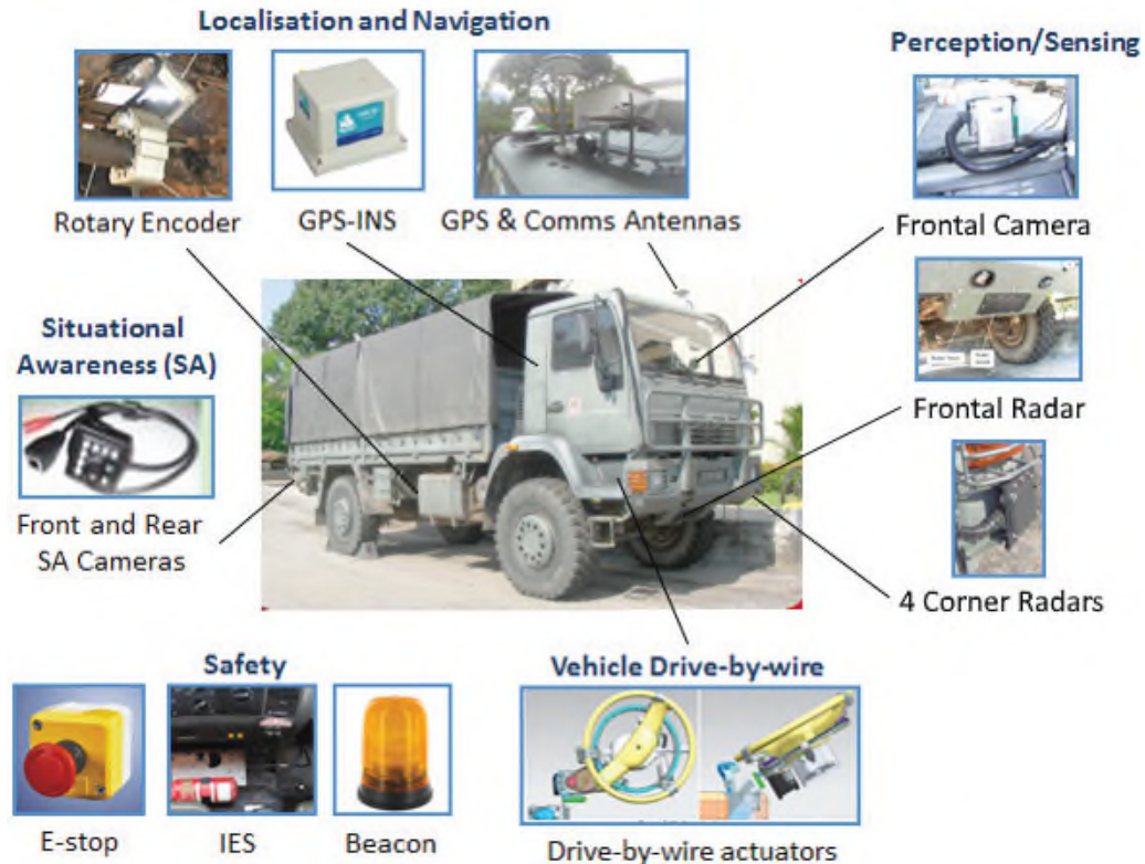
Figure 3. Main hardware subsystems installed in the Unmanned Follower (Reprinted with permission from ST Engineering)
