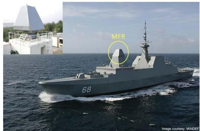
Figure 8. MFR on board the frigate (MINDEF, n.d.)
