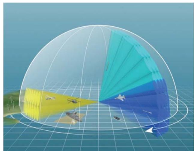
Figure 10. Dual-axis multi-beam. An individual colour illustrates a transmit beam with simultaneous receive beams
