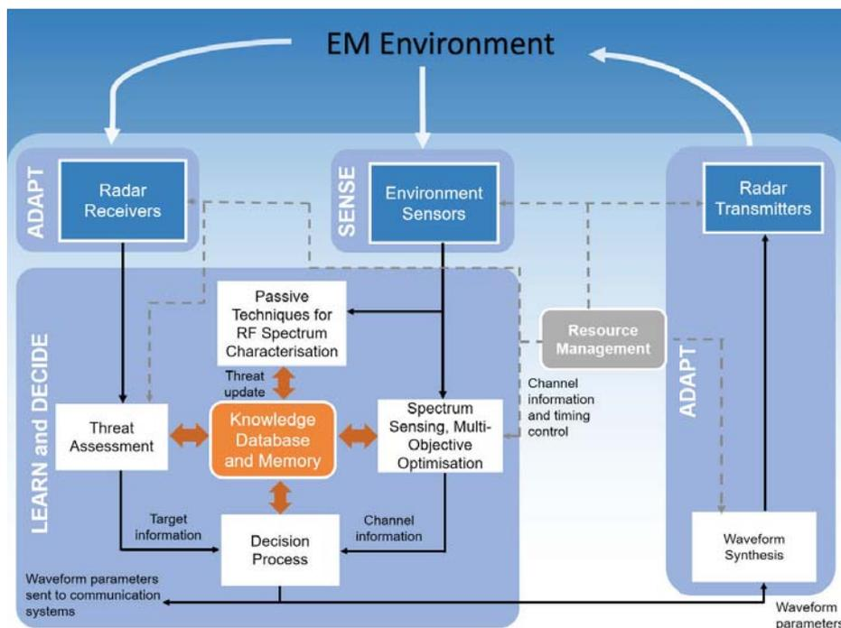
Figure 16. A cognitive radar architecture for operating in congested and dynamic EM environment
