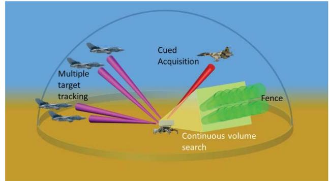
Figure 7. Various functions of a multi-function radar
