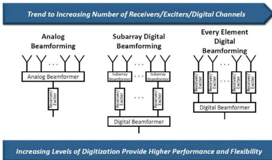
Figure 13. Trend in beamforming, from analog to digital (SAAB, n.d.)
