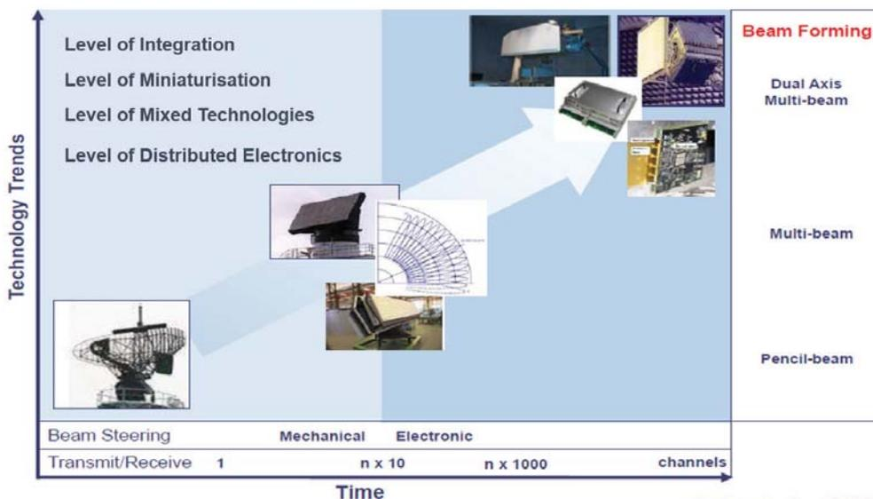
Figure 9. Trends in antenna architecture and beamforming
