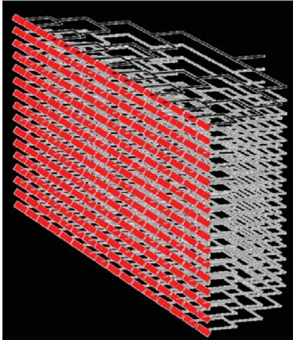
Figure 6. Stack of individual stripline array
