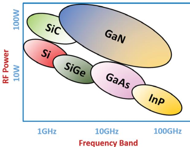
Figure 15. RF power versus frequency for major semiconductor devices
