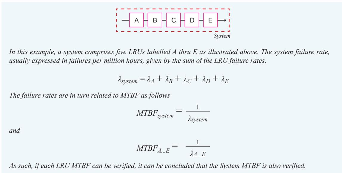
Figure 3. System MTBF and LRU MTBF in reliability verification
