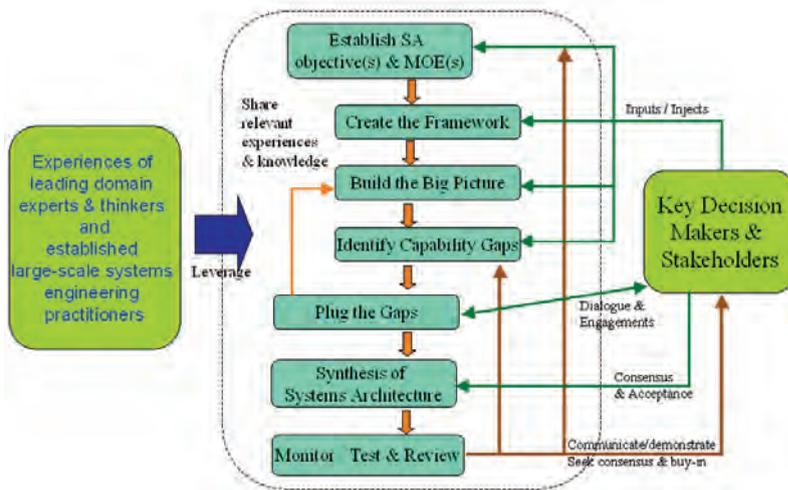
Figure 5. A seven-step methodology for Systems Architecting
