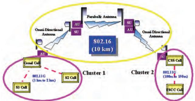
Figure 3. D-Hub Configuration for a 10km Brigade CP footprint
