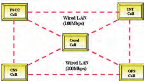
Figure 2. Centralised CP Configuration
