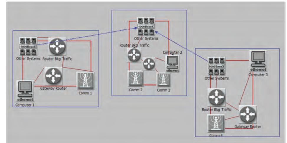
Figure 2. Communications network simulation environment using OPNET Modeler
