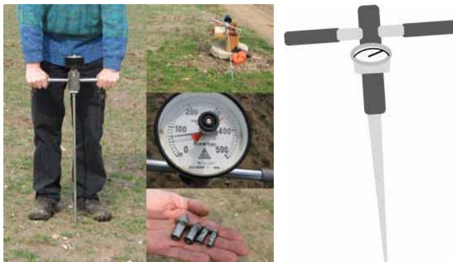
Figure 3. Cone Penetrometer (© HPsy / File:Penetrometer.jpg / <https://commons.wikimedia.org/wiki/File:Penetrometer.jpg> / Public Domain)
